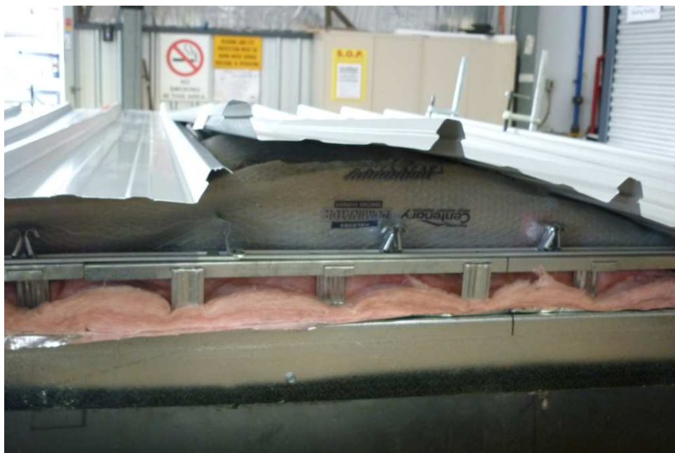
Figure 7. Separation of centre test panel from side panels at overlaps at failure.
