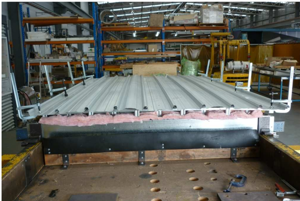
Figure 5. Deflection of the sheet at airbag pressure of 7.68kPa.
