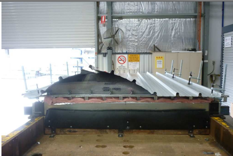
Figure 6. Sheeting at failure.
