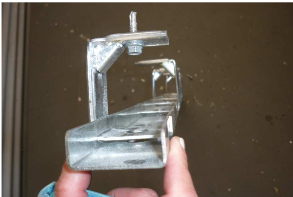
Figure 6. No permanent damage at the spacer after testing.
