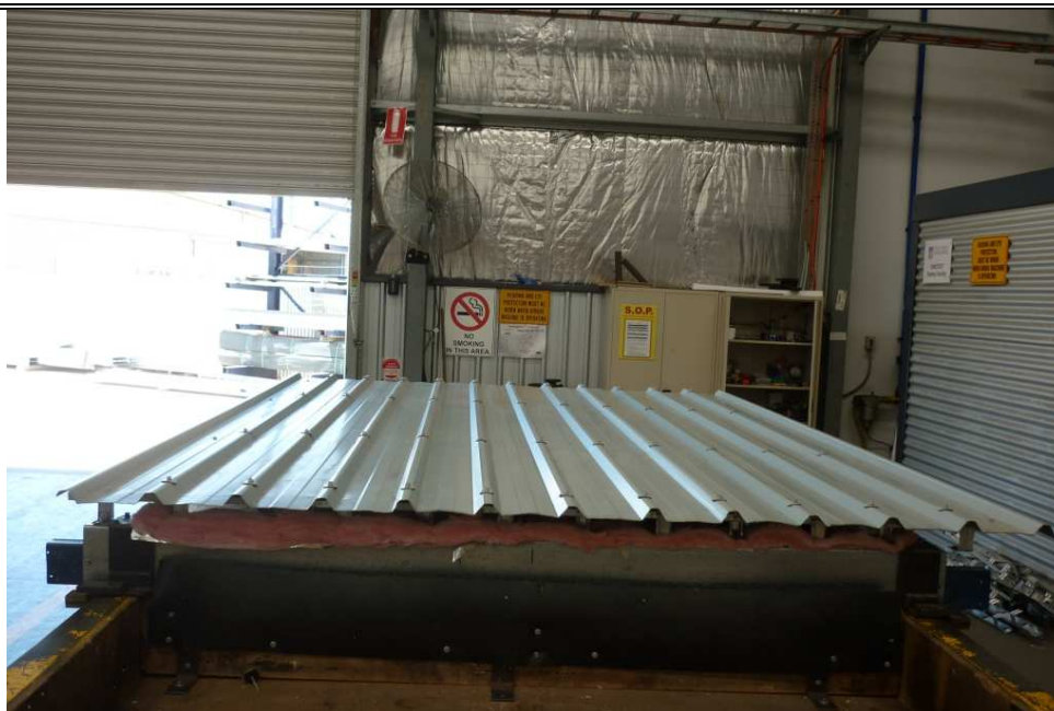
Figure 2. Installed sheet prior to testing.
